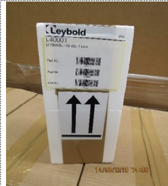
Example LVO 400: Packaging of a glass bottle in polystyrene and adhesive tape.
