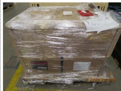
Packaging example cartons on Euro pallet with stretch film and edge protection.
